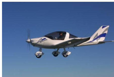
The sting aircraft in cruise configuration, 125 kn for around 15 L per hour
