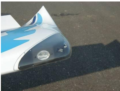
Integrated landing light, strobe and navigation beacon can be fitted to each wing tip
