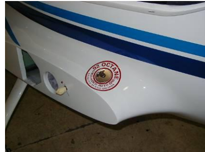
Flush mounted fuel filler caps eliminate problems with drag
