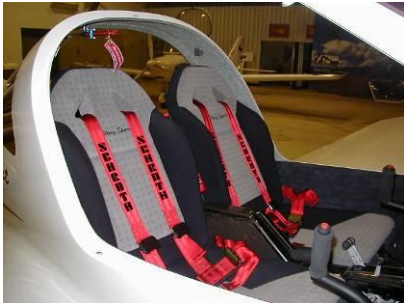
Comfortable bucket seats firmly hold the pilot and passenger in the aircraft
