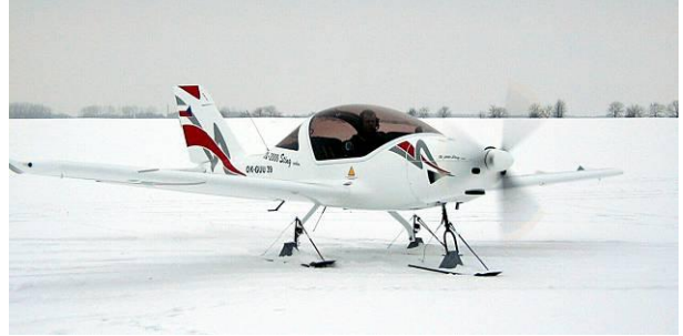
Sting aircraft can be successfully operated of snow skis
