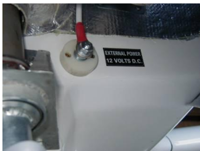
The sting is a mature design, here is the external battery connection if you ever need to jumpstart your aircraft
